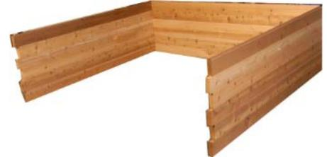
Step 2: put in place the second level panels in the same sequence as the bottom panels. Before putting in place, run a bead of Tite-Bond glue along the tongue on the top board of the bottom panels. Bench brackets are pre-mounted on the specific panels - this must be considered so that the correct panels are positioned in their correct location.
