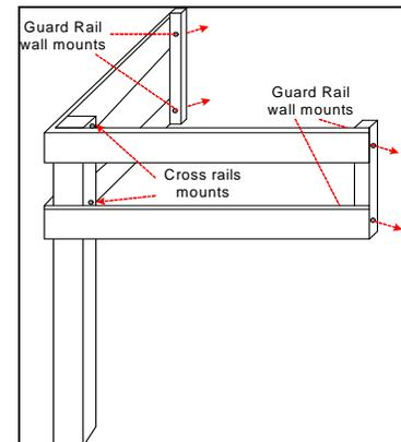
Step 12: Heater guard rails need minor assembly. First - mount the cross rails to the primary corner post. These holes are pre-drilled and they need to be drilled from the back. Once assembled, position the guard rail with proper distancing from the heater. Make sure railings are square. Drill the guard rail into the wall with supplied screws.
